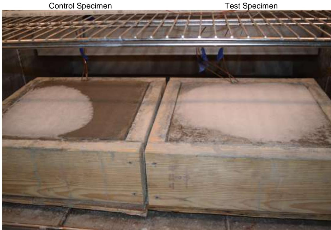
\*The test specimen has evidence of ice and frost on the surface while the control specimen has absorbed the moisture.
