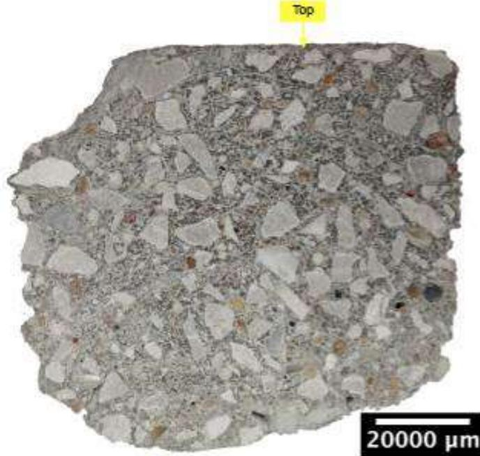
Control Specimen (Unreated) – Slab View
