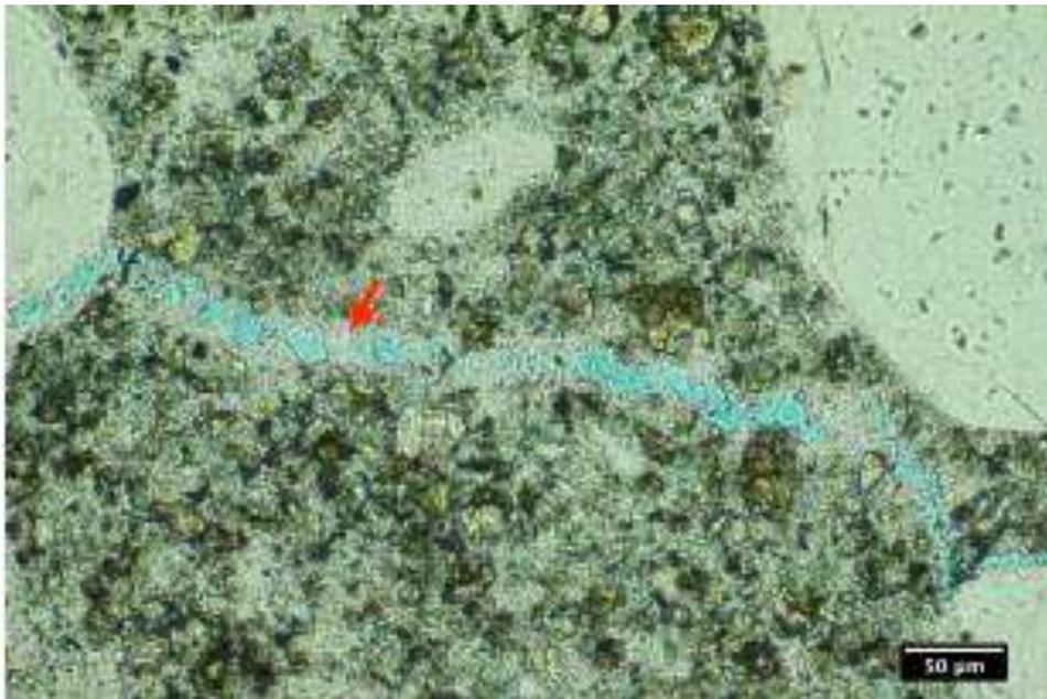
Fracture-bridging calcite cement (red arrows). Note the diffuse & microporous character of the cement paste.
