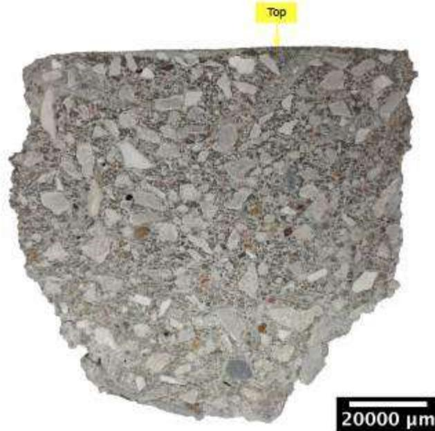
Test Specimen (Treated) – Petrographic Thin Section
